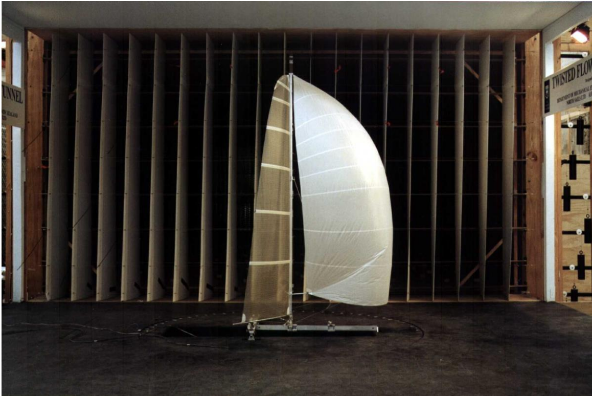
Figure 1. Model mainsail and spinnaker sails under test in the University of Auckland Twisted Flow Wind Tunnel.
