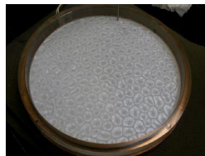
Figure 13: Photo of Rayleigh-Bénard experimental set up with a free upper surface (From John Matsson, thesis).
