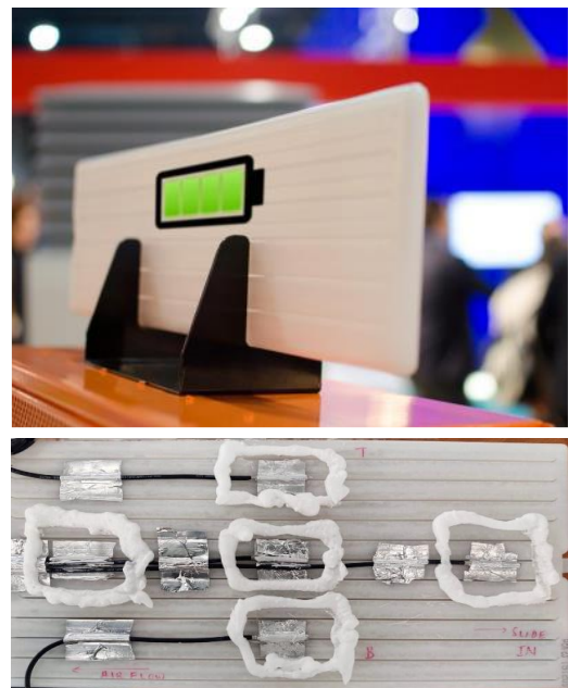
(c) PCM-panels, temperature sensors are connected on the lowest panel surface.
