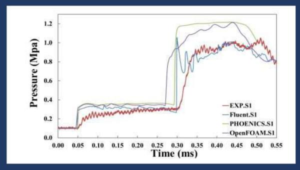
Fig.5 Micro shock-tube: Measured and Predicted pressure histories at the Sensor S1.
