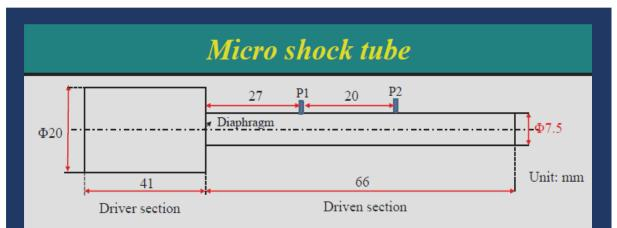
Fig.1 Schematic of the closed micro shock tube
