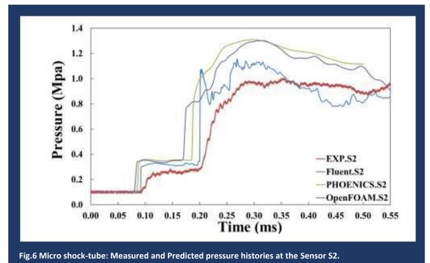
Further work is needed to investigate the reasons for the discrepancies between the three codes and experiment.
